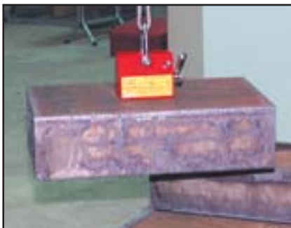
Center magnet on most workpieces to lift.
