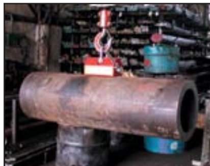
Beveled bottom surface lifts round stock.
