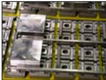
Machine induction blocks to create work-stops for fast, accurate part alignment when ganging parts together for repeat jobs.
