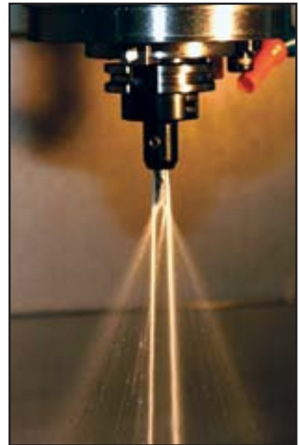
CoolBLAST in-the-bore coolant ports blast coolant on the tool path, even at high RPMs.
