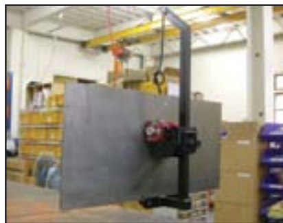
Vertical Lifters can be operated by one person.
