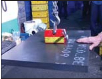
Safest way to move ferrous stock.
