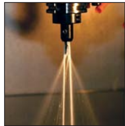
CoolBLAST in-the-bore coolant ports blast coolant on the tool path, even at high RPMs.
