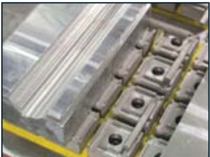
Use induction blocks as work stops
