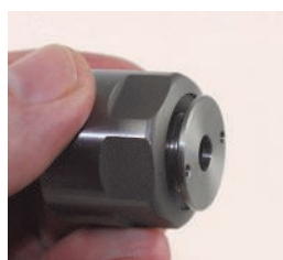
Thread Coolant Cap into TG nut, snug with wrench after the collet has been assembled.
