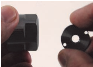
Thread Coolant Cap into SX nut, snug with wrench after the collet has been assembled.
