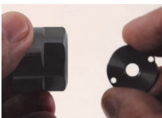
Thread Coolant Cap into TG nut, snug with wrench after the collet has been assembled.
