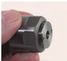
Thread Coolant Cap into SX nut, snug with wrench after the collet has been assembled.
