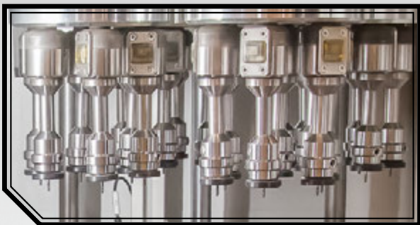
4 on-site Otec Post Polish machines
