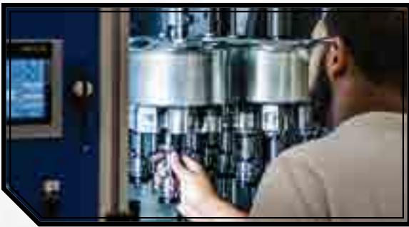
3 on-site Otec Post Polish machines
