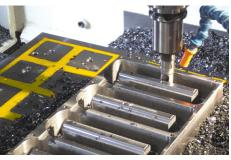
Machining mold cavities
