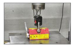
**3. Testing:** A Load test is performed, confirming your magnet meets its required load capacity, and is certified in compliance with ASME B30.2.
