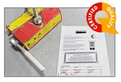
**4. Certification:** Results are recorded and a Certificate of Compliance is prepared and shipped back to you with your repaired magnet.
